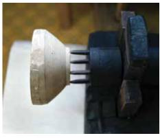
A bowl blank tapped onto pins so the interior could be hollowed.
